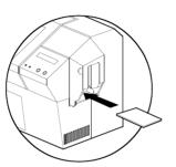
For one-at-a-time printing, feed cards through slot on side of Feeder.
